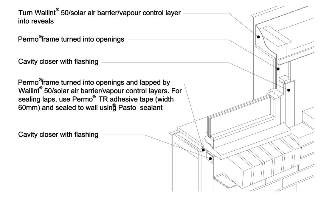
TYPICAL PERMO<sup>®</sup> FRAME INSTALLATION DETAIL DRG No. KL006
